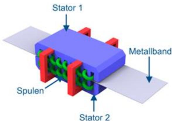
*Schematic representation: The contact-free feed process adopts the principle of magnetic attraction and repulsion. Two stators make this possible by generating a traveling magnetic wave in the metal strip.*
